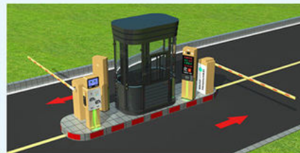
Two Lanes : One Entrance + One Exit (SEWO CP9 + Ticket Parking Equipment)
